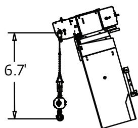
Dimensions are for largest furnished hookblock and headache ball with anti-two block activated.
